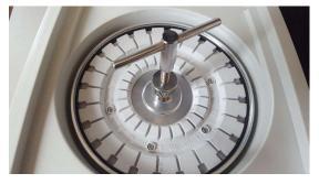
4. Once the removal tool is securely screwed onto the rotor, begin to turn the removal tool handle clockwisewhile holding the rotor at the same time so that the rotor does not move while turning the handle.
