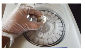
2. Get the rotor removal tool and turn the handle anti-clockwise so that the centre pin goes further inside.
