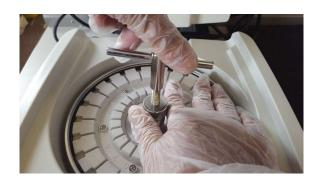
5. While turning the removal tool handle clockwise, the rotor should start to lift away from the motor shaft, once the rotor is free from the motor shaft, the rotor can now be removed by pulling rotor upwards by theremoval tool handle.
