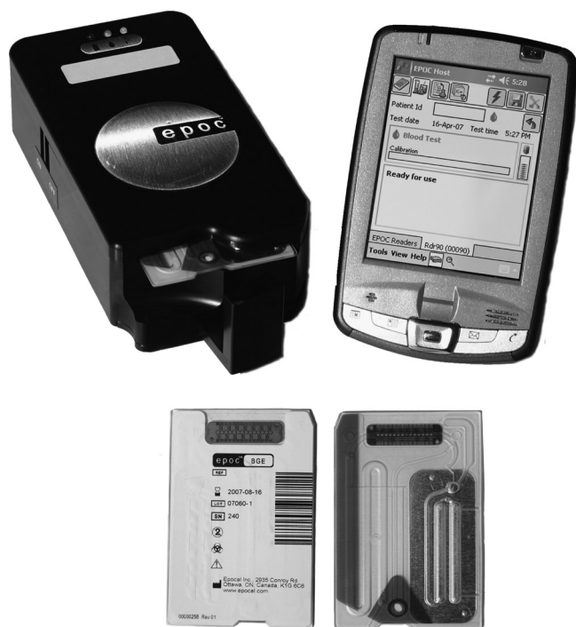
FIGURE 1. The EPOC system. The EPOC blood analysis system consists of individual test cards (front and back of card in lower half of figure) that can provide blood gas and electrolyte analysis in multiple configurations. This configuration uses a card reader (upper left) that detects signals from the biosensor on the test card and transmits the data wirelessly to a handheld PDA that contains the EPOC software to calculate analyte concentration from the raw card signals. Other configurations allow the card reader to wirelessly connect to PCs or other hardware running the EPOC software.
