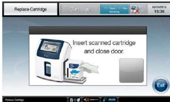
8. Facing the cartridge label, insert the cartridge into the analyzer.
