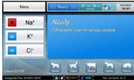
2. Press the **Sensor Status** icon twice quickly. The latest slope result of the sensor and the allowable slope range will appear.
