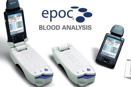
The epoc, developed by the founder of the i-STAT analyser, is the first wireless point of care testing solution to use Smart Card technology. The epoc provides immediate blood gas, electrolyte and critical care biochemistry results directly to a hand held pda (included) and wirelessly interfaces to an electronic data manager (EDM) and bluetooth printer. It is a completely
